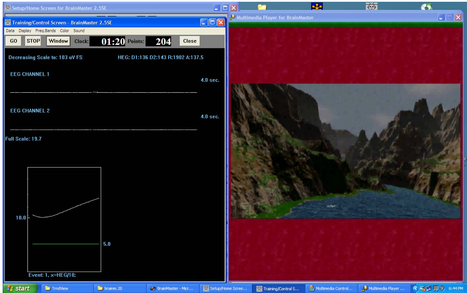
BrainMaster HEG with MMP Multimedia Player. Animation moves and music plays whenever signal rises.
