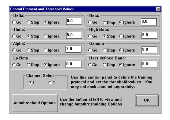
This screen is used to customize the protocol so that the EEG signal can be used to control the computer. Each of the frequency components can be set to either "Go", "Stop", or "Ignore." The user may select the desired combination of control rules by using the "radio" buttons associated with each component. If a study protocol has been selected from the trainee/study screen using the "Restore Settings" button, then the screen will display the preset information.
