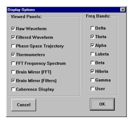
This screen selects the various screens that will appear in the "client area" of the "Master" program. These settings are saved and restored to the sessions file, and are sent to the "Master" module through the DLL interface. In addition to each display window, it is possible to select which frequency bands are reflected in the thermometers, plots, and other displays.
