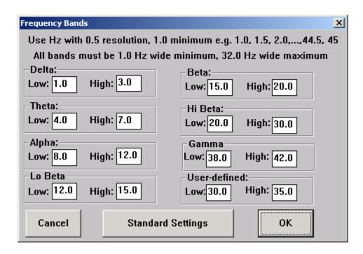
This is the Frequency Bands control screen. It sets the frequency range of the digital filters, and the FFT analysis, by setting the low and high cutoffs for each defined band.
