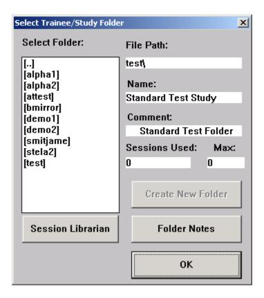
This screen allows the user to select the current folder and also provides the ability to create a new folder. A folder can be selected by scrolling in the list below the "Select Folder" label and clicking on a desired trainee. The trainee's name and directory are immediately displayed. This trainee is automatically selected and will automatically default as the current trainee the next time the "Master" program is run.
