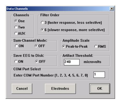
The Data Channels screen allows the user to configure the following items:
