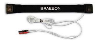
This Respiratory Effort Sensor includes a transducer with two standard "touch-proof" connectors. The device produces an output voltage that is proportional to respiratory effort, and which can be read into the Atlantis device using the "DC" mode of the amplifiers. It is possible to plug this sensor directly into the Atlantis EEG inputs, and use its output for training, as described below.
