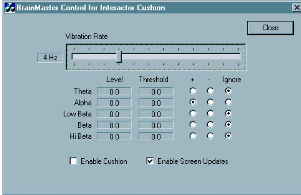
The “Vibration Rate” control sets the rate at which the cushion will vibrate. This can be set from 1 vibration per second, to 12 vibrations per second.
